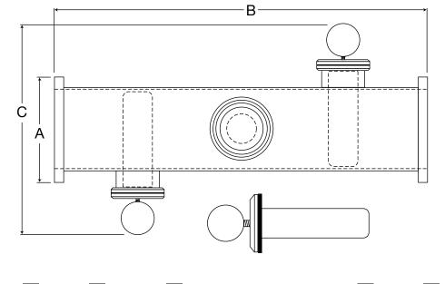
**Note:** Maximum pressure rating for 70°F. Each liquid trap is tested to 150% of rated pressure. MLT's are NOT ASME CODE certified. Before ordering, check local and state pressure vessel requirements.
